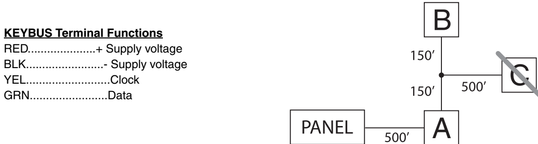
Figure 3.2: KEYBUS Wiring
